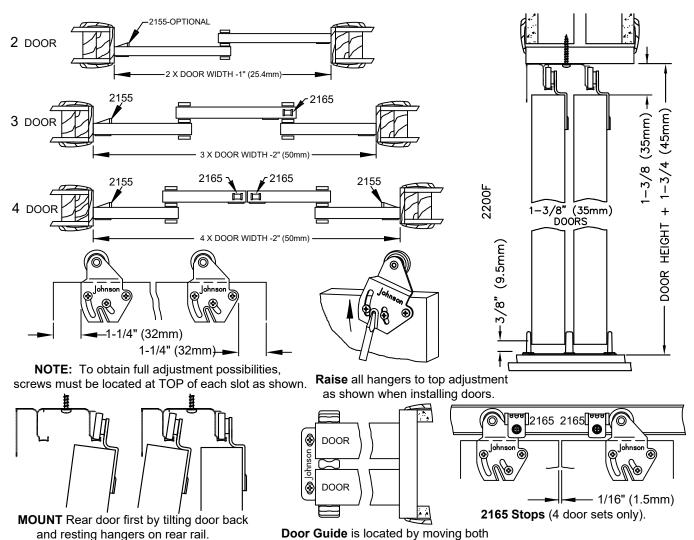
MOUNT Front door the same way by tilting back and placing hangers on front rail.
