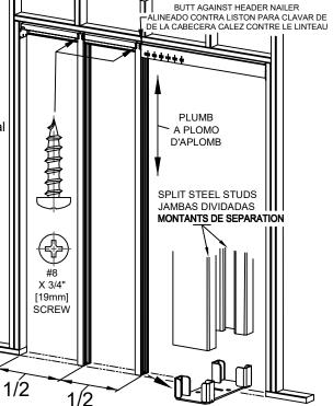
**6** Apply desired wall material with 1" (25.4mm) X #6 Self drilling drywall screws. Use seven (7) screws per Split Steel Stud.
