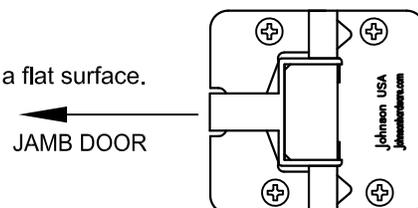
**3 FASTEN PIVOT PLATES** to top and bottom of doors as shown.
