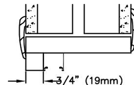
**2 MOUNT HINGES (1703) on back of door. Lay panels face down on a flat surface.**
