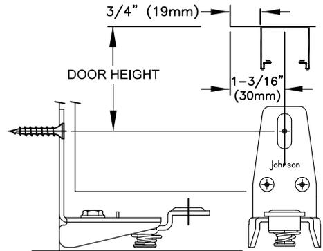
**5 HANG DOORS:** Make sure Track Pivot Lock (1710) is in the unlocked position. (A) Fold doors and insert 1705 into track groove. Place 1701 into receptor of 1710. (B) When firmly seated, slide tab lock toward pin. Door now should be hanging from 1701. (C) Depress 1711 pivot socket arm and insert 1707. If no vertical adjustment is needed, secure 1711 with other 2 screws. Use 1712 wrench for horizontal adjustment of 1710 and 1711.
