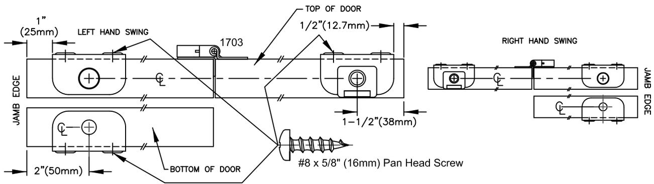
**4 MARK LOCATION** of Jamb Bracket (1711) on jamb. Fasten 1711 in place with one #8 X 1-1/4" (32mm) flat head screw.
