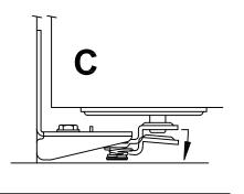
ADJUST SNUBBER (1713) Close doors, slide 1713 until it touches 1705. Open doors, move 1713 1/8" (3mm) closer to 1705 and tighten. Doors should "snap" shut yet open easily by a slight pull on the knob.
