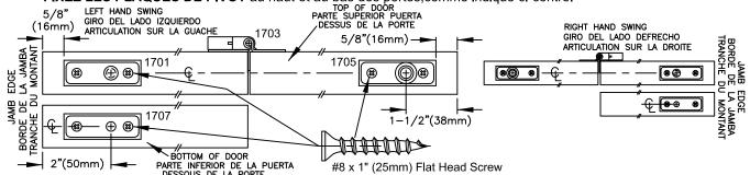
MARK LOCATION of Jamb Bracket (1711) on jamb. Fasten 1711 in place with one #8 X 1-1/4" (32mm) flat head screw.
