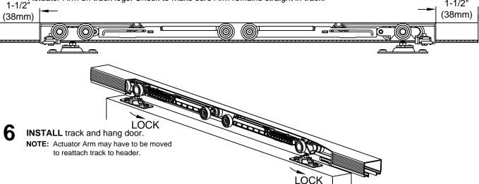
**SLOWLY** slide door toward Jambs, checking to make sure door touches Jamb, if not. Slide door away from Jamb and readjust Actuator Arm. Slowly close door again, checking to make sure soft close is working properly. Once confirmed, begin using door normally.
